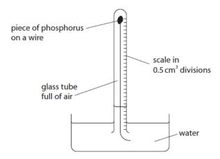
The volume of gas in the tube decreases as the phosphorus reacts with oxygen. The teacher measures the volume of gas in the tube at one-minute intervals. The table shows the teacher's results.
